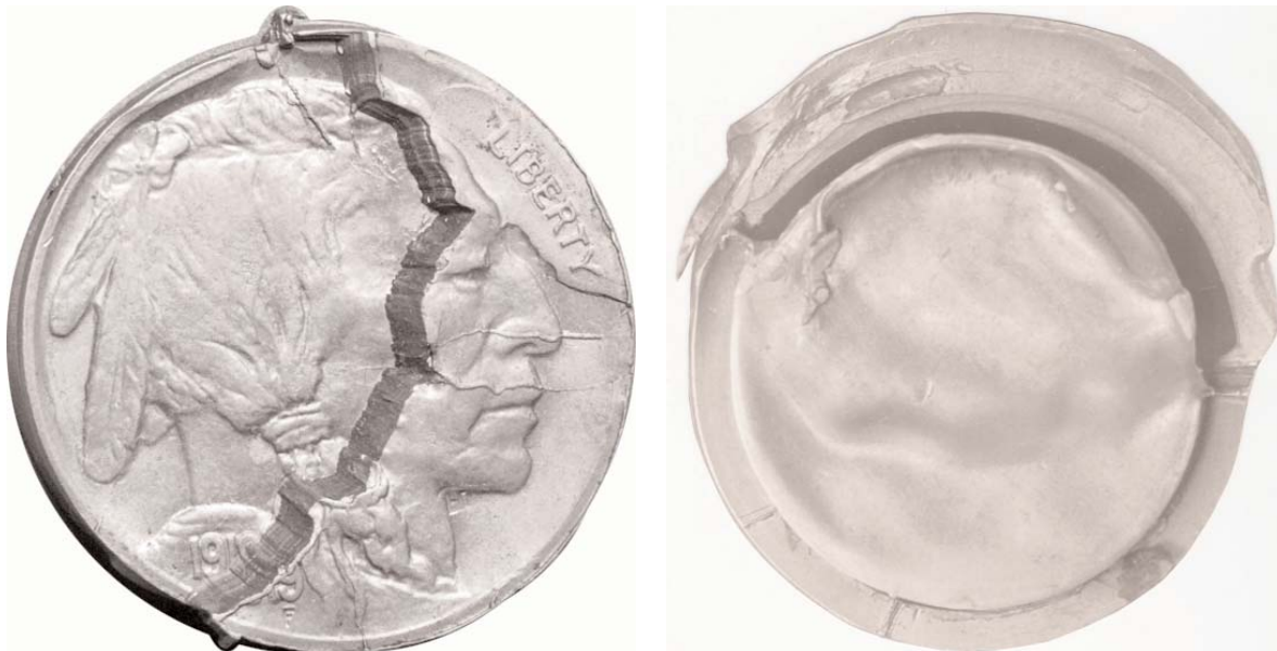
Figure 10a,b. Catastrophic die failure of the obverse (anvil) die in a multi-struck 1919 buffalo nickel. A huge retained cud with extreme vertical displacement stands amidst a profusion of die cracks. The whole business is surrounded by a broken collar. Photos courtesy of Ken Hill.
