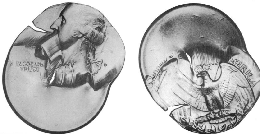
Figures 9c,d. Second coin. Most of the remaining portion of the obverse face broke away at the moment of the strike, stretching out the planchet. The only intact part of the die face left is a small corner incorporating Washington's chin and IN GOD WE TRUST. Severe clash marks are present on both faces.
