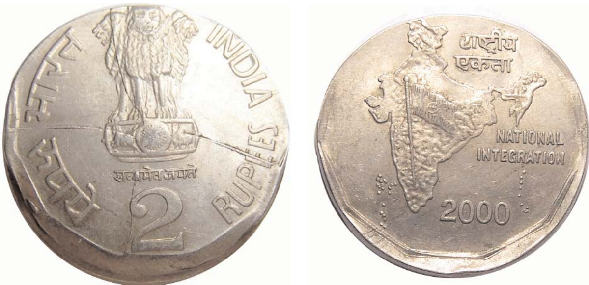
Figure 3a,b. A 2000 Indian 2 rupees coin with four severe bi-level die cracks converging on the center of the coin. Photos courtesy of Jeff Ylitalo.
