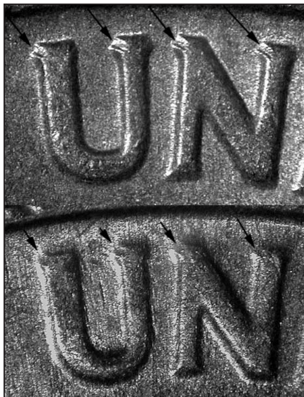
Comparison of EDS (above images) and LDS examples of 1964-D 1c DDR012 highlight the marked difference in notching as the die wears.
