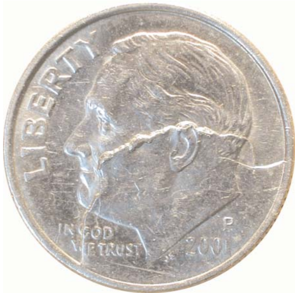
Figure 6a. A 2001b dime with a huge retained cud and three bi-level die cracks. The reverse is normal.
