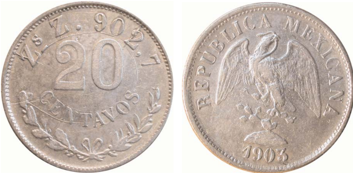
Figure 2a, b. A 1903 Mexican 20 centavos struck by a shattered reverse die. Numerous radial and curved die cracks have spread across the reverse face.
