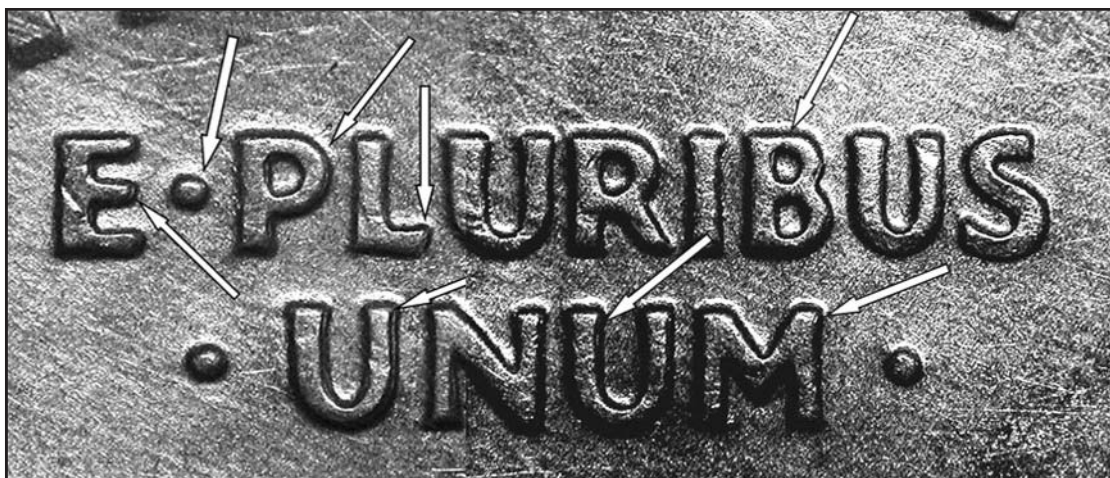
Figure 1: 2003-D Lincoln cent submitted by Bill Slaughter appears to have the same type doubling as the 2004-D Lincoln cents. It being a Class IV + VIII doubled die with medium spread on the lettering and the periods.
