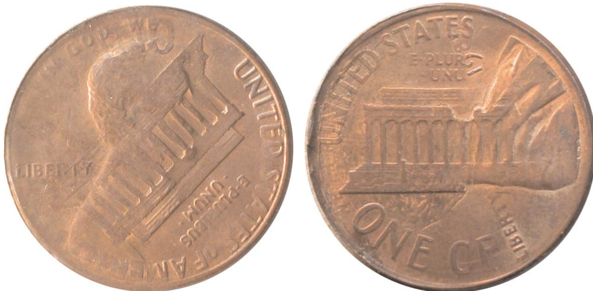
Figure 1a,b. A 1985 cent with what appears to be a flipover, in-collar double-strike. The second strike shows a massive vertical misalignment (tilted die error). The photos are oriented so that the second strike is in the upright position. Coin on loan from Fred Weinberg.
