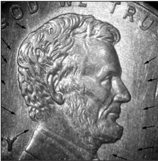
Obverse die mated with Stage "B" reverse of 1999P-1DER-015WS bears many fine die scratches.
