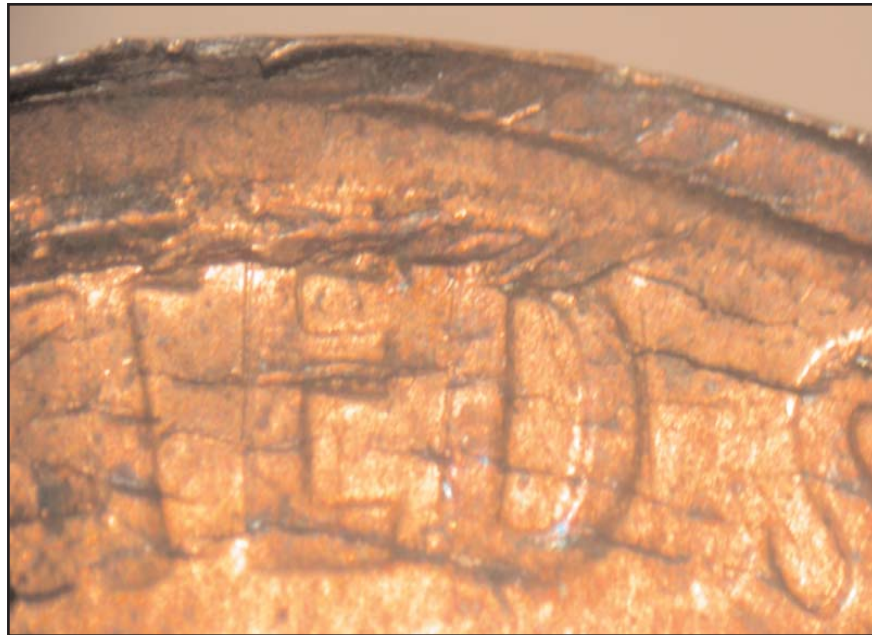
Figure 5. Close-up of UNITED from the second strike. The letters show abnormally low relief and look like they've been flattened. The copper plating in this area appears cracked and buckled and there is a profusion of strange raised lines. Note how the surface of the coin slopes gradually upward toward a sharp, elevated margin. There is no design rim here.
