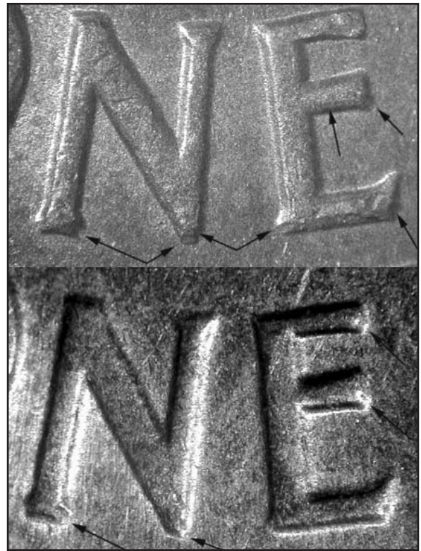
Notching of the letter C on the LDS coin (bottom images) has been completely obliterated by die wear. Notching visible on NE of ONE has been severely degraded.
