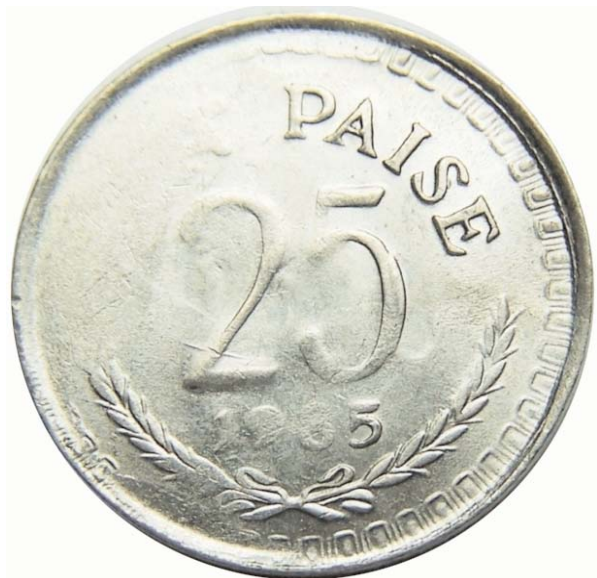
Figure 8d. Reverse face showing numerous weakly struck areas. The largest and most profound area of weakness (upper left side) was due to a tilted die, which, in turn, was probably caused by a broken die base or shaft.
