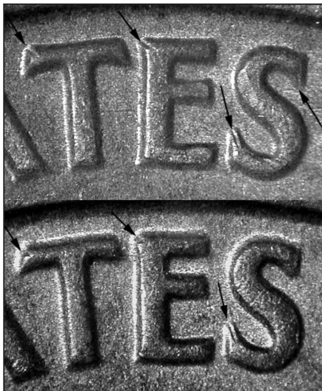
Comparison of EDS (above images) and LDS examples of 1964-D 1c DDR012 highlight the marked difference in notching as the die wears.
