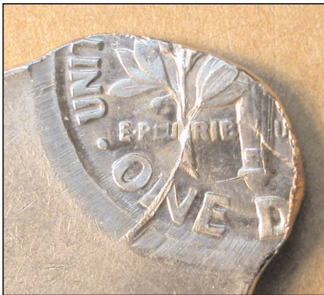
Figure 11a,b. Double-struck dime with the larger strike showing a shattered reverse die. Numerous bi-level die cracks cross a surface covered with multiple sets of clash marks. The obverse face shows such heavy, closely-spaced clashing that the individual clash marks are blurred, along with the low-lying parts of the design. The smaller strike was delivered by a tiny portion of an obverse die. It was delivered at an angle of approximately 45 degrees. See text for further details.
