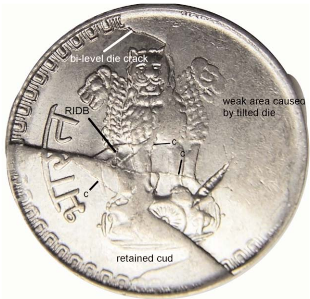
Figure 8a,b. A 1985 Indian 25 paise coin showing various types of brittle fracture, that, in aggregate, elevate it to the level of a shattered die. Abbreviations: RIDB, retained interior die break; c, die crack; other labels are self-explanatory. Photos courtesy of Jeff Ylitalo.
