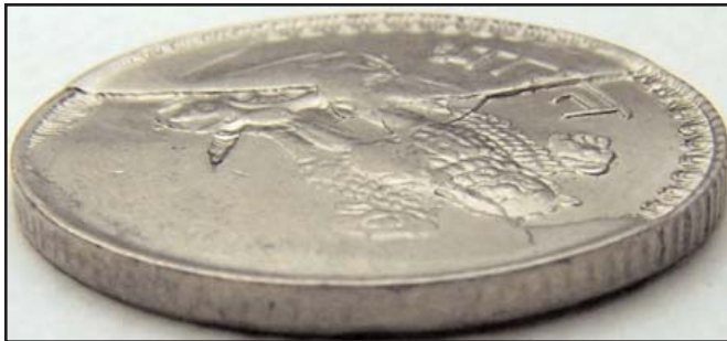
Figure 8c. Oblique view showing vertical displacement at the edge of the retained cud.
