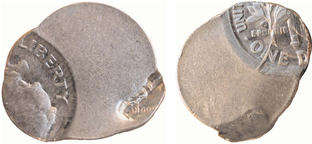
Figure 11a,b. Double-struck dime with the larger strike showing a shattered reverse die. Numerous bi-level die cracks cross a surface covered with multiple sets of clash marks. The obverse face shows such heavy, closely-spaced clashing that the individual clash marks are blurred, along with the low-lying parts of the design. The smaller strike was delivered by a tiny portion of an obverse die. It was delivered at an angle of approximately 45 degrees. See text for further details.
