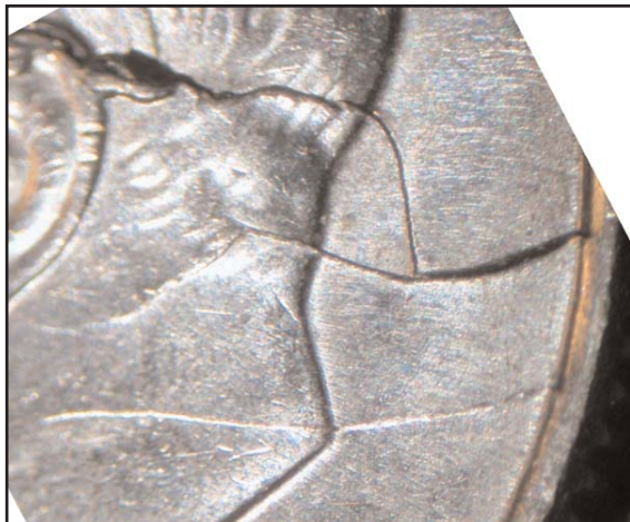
Figure 6c. Two bilevel die cracks appear on the right, one of which extends in from the retained cud, the other extending in from the rim.
