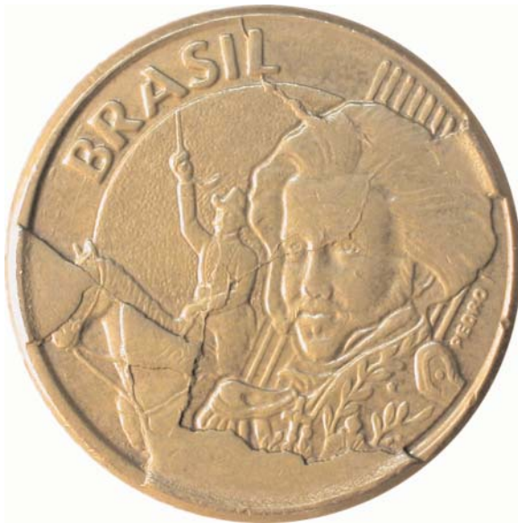
Figure 7a,b. Obverse face of a 2002 Brazilian 10 centavos with various manifestations of brittle fracture. Abbreviations: RIDB, retained interior die break; c, die crack; other labels are self-explanatory.
