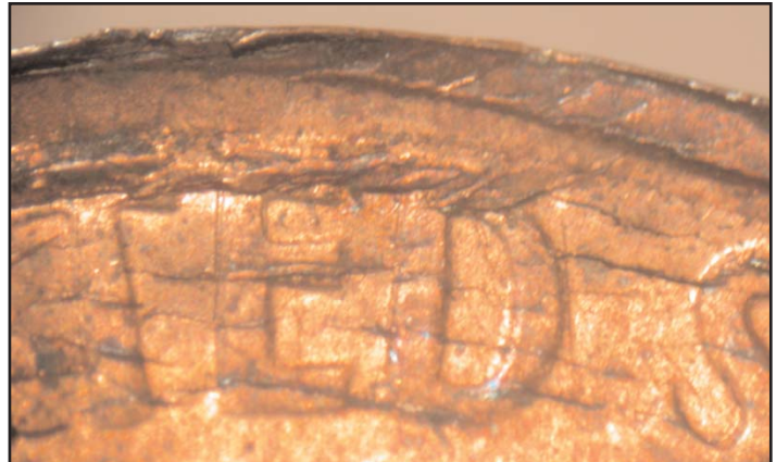
Figure 6. Extreme close-up of UNITED showing the many short, gently curved ridges that parallel the perimeter of the coin. The plating is cracked here and the exposed zinc appears to have oxidized.
