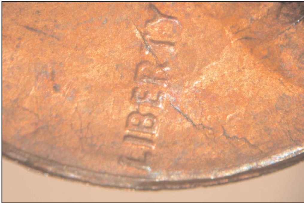
Figure 8. A close-up of the area around and below LIBERTY of the second strike, showing a leathery texture and a pattern of cracking and crazing.
