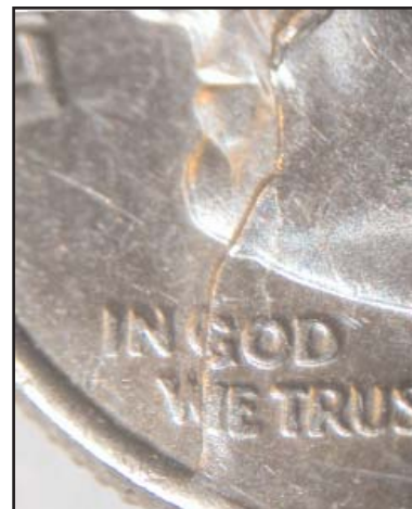
Figure 6d. Close-up of a small bi-level die crack extending from the retained cud and passing through the "O" of GOD. Significant horizontal offset is seen at the edge of the retained cud in this area.
