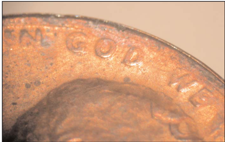
Figure 3. A close-up of IN GOD WE TRUST from the second strike. The letters show low relief and are somewhat indistinct. The “I” of IN is especially faint.
