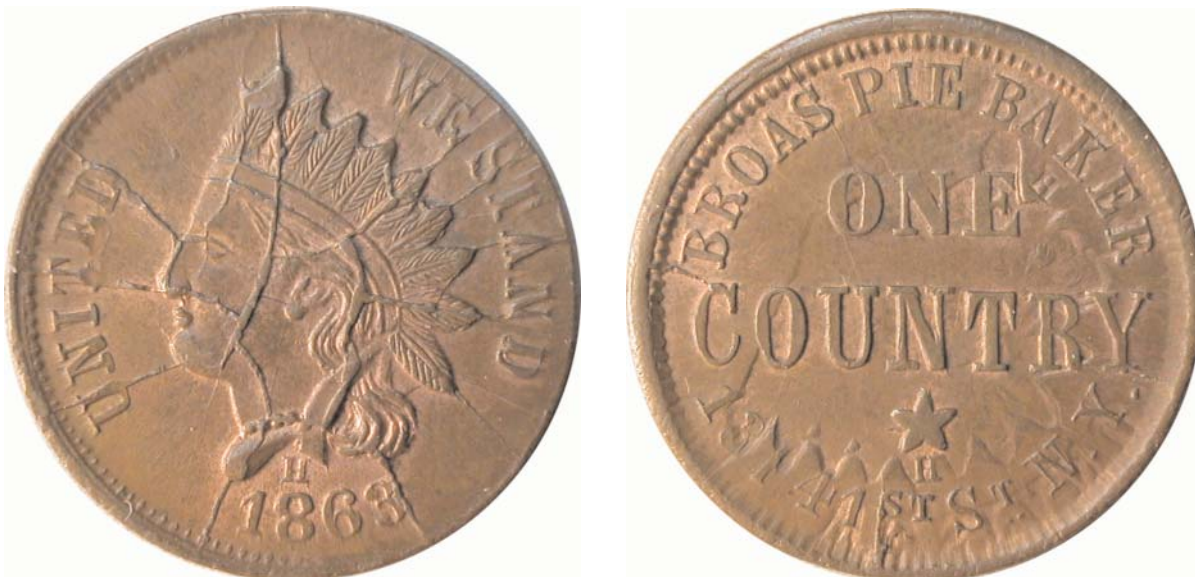
Figure 5a, b. An 1863 Civil War token struck by a shattered obverse die. A large number of thick radial die cracks converge on a centrally located circular die crack. The pattern resembles the hub and spokes of a bicycle wheel. Severe clash marks on the reverse seem unrelated to the fractured surface of the opposing die.
