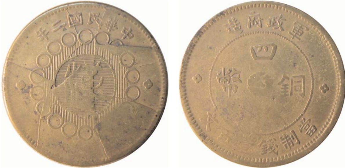
Figure 4a,b. A 1913 Chinese 100 cash coin with numerous intersecting bi-level die cracks. The cracks divide the obverse face into blocks of different height.
