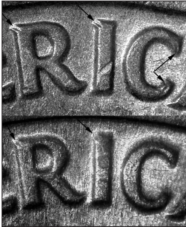
Notching of the letter C on the LDS coin (bottom images) has been completely obliterated by die wear. Notching visible on NE of ONE has been severely degraded.
