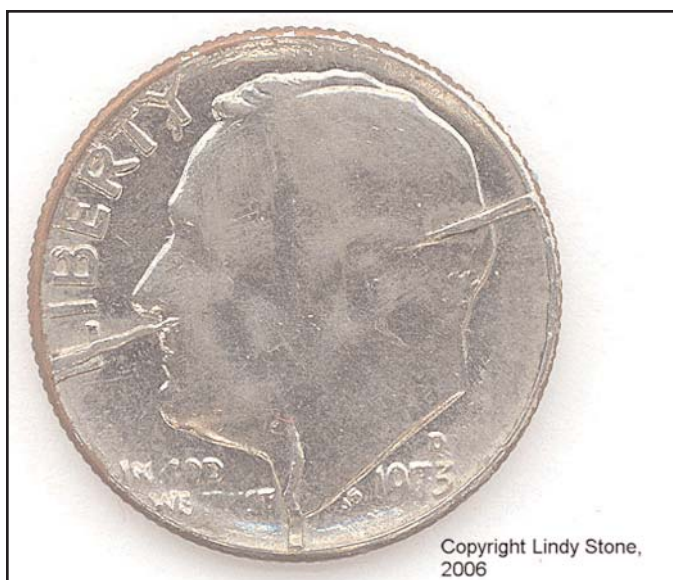
Figure 1. A 1973-D dime struck by a shattered obverse die. The die face shows a full split and a half-split in the southern hemisphere. Photo courtesy of Lindy Stone.
