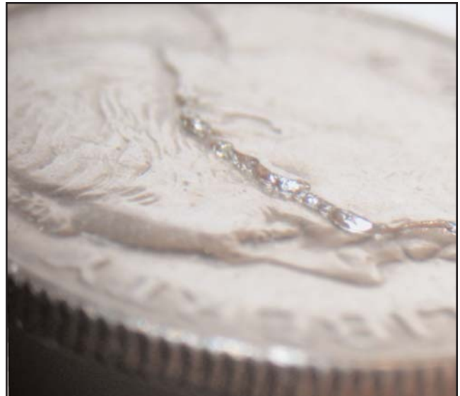
Figure 6b. Oblique view of the retained cud showing dramatic vertical displacement.
