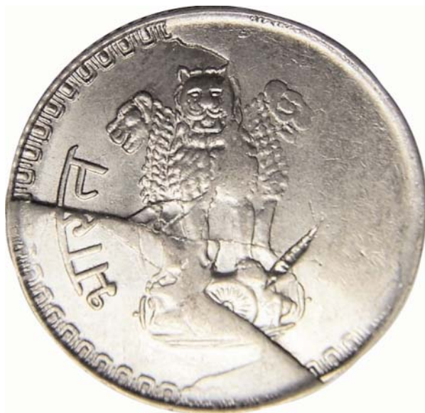
Figure 8a,b. A 1985 Indian 25 paise coin showing various types of brittle fracture, that, in aggregate, elevate it to the level of a shattered die. Abbreviations: RIDB, retained interior die break; c, die crack; other labels are self-explanatory. Photos courtesy of Jeff Ylitalo.
