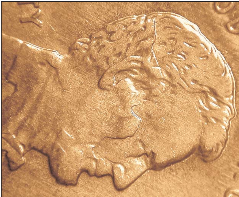
Closeup images of the double strike show the extent of rotation of the coin between strikes. Images courtesy BJ Neff.
