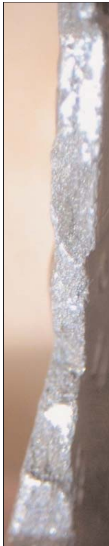
Alfonso Chio's 1962 nickel was struck on an extremely brittle planchet that fractured during and/or after the strike.
