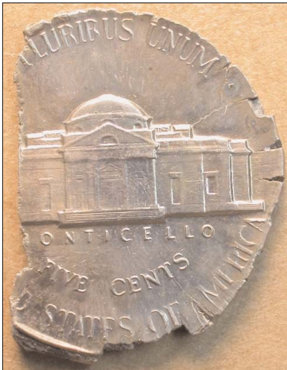
Alfonso Chio's 1962 nickel was struck on an extremely brittle planchet that fractured during and/or after the strike.
