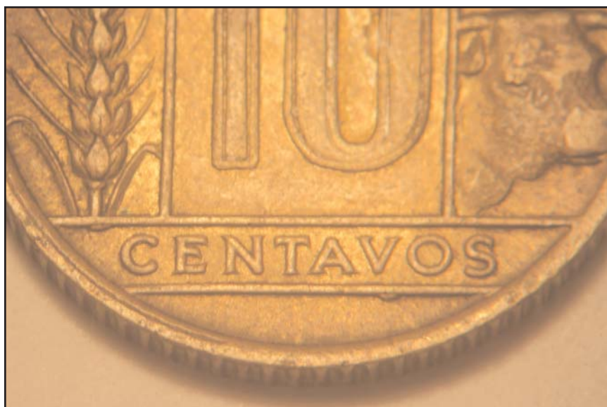
Argentina 1944 10 Centavos with die chips above and to right of C in CENTAVOS and below V of CENTAVOS.
