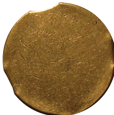
Nickel Blank Planchet, Type II, Triple Curved Clipped 2-4% - Other Side
