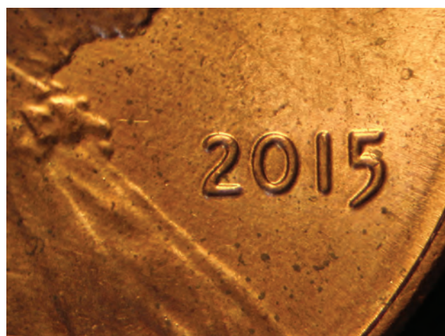
2015 Lincoln Cent bisecting die crack
