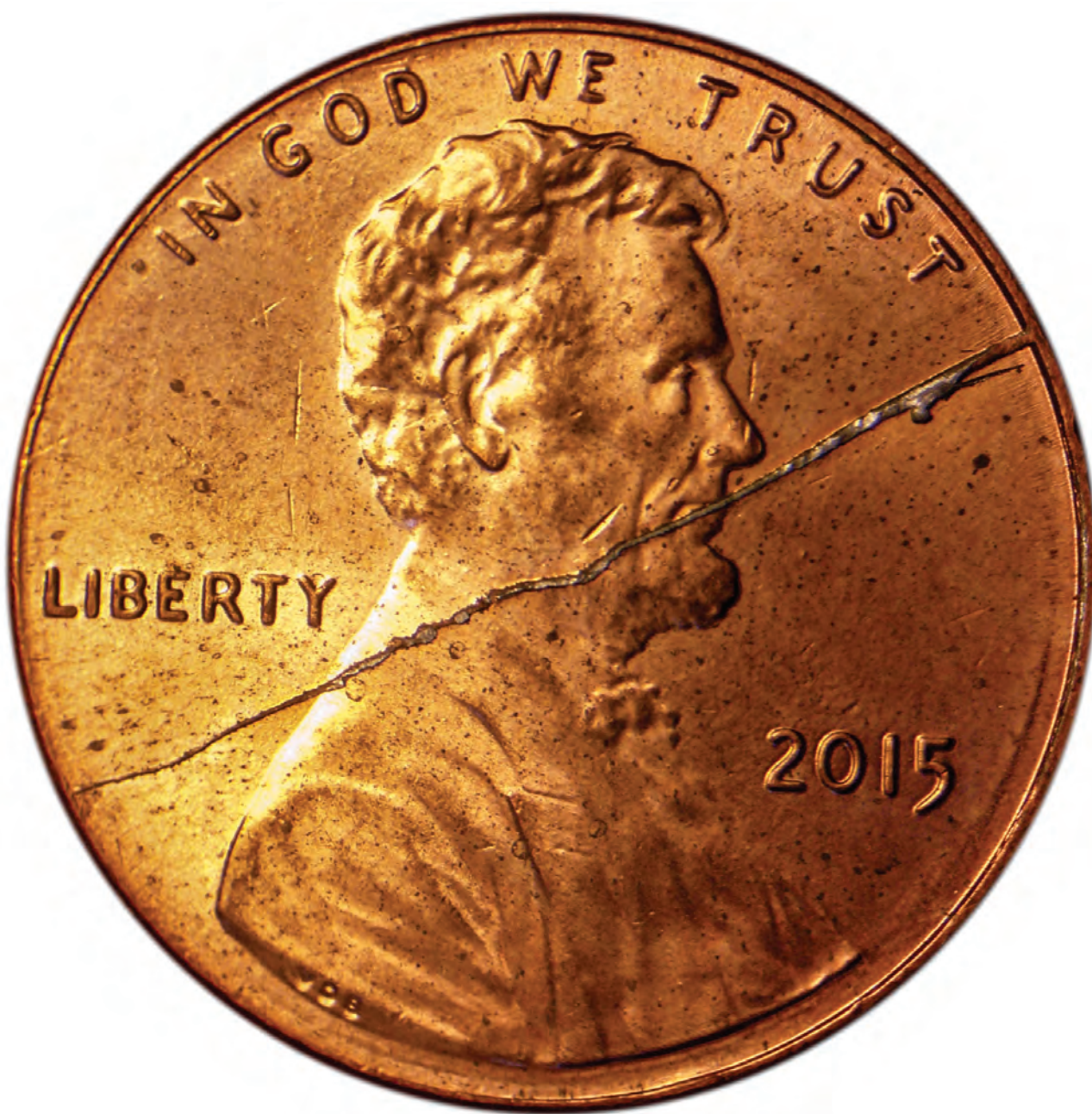
2015 Lincoln Cent bisecting die crack
